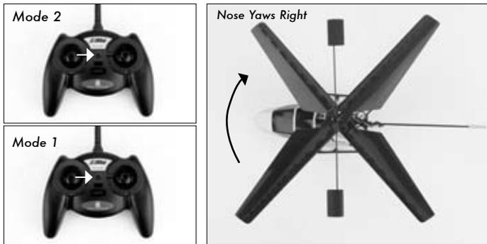
The rudder trim can be used to help keep the nose of the helicopter from rotating to the left or right when in hover with no rudder stick input. For example, if the nose of the helicopter drifts to the right when in hover, add left rudder trim (by pressing the left rudder trim button) until the nose stays as close to straight as possible.
