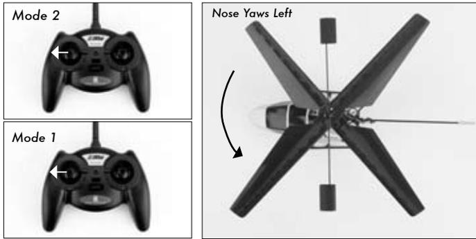
Moving the stick to the right will turn (yaw) the nose of the helicopter to the right about the axis of the main shaft. This is accomplished by increasing the speed of the upper main rotor blade while decreasing the speed of the lower main rotor blade.
