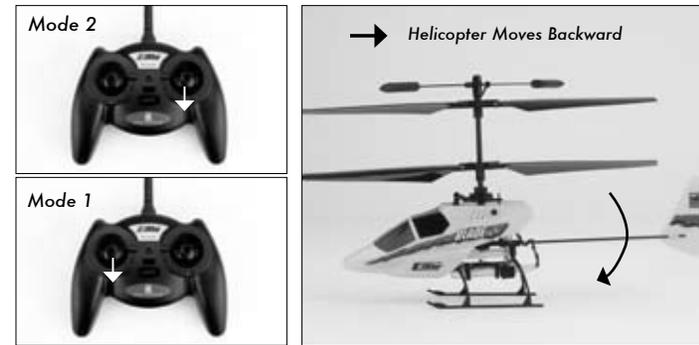
The elevator trim can be used to help keep the helicopter from drifting forward or backward when in hover with no elevator stick input. For example, if the helicopter drifts forward when in hover, add back/up elevator trim until the helicopter hovers as level as possible with no forward drifting.
