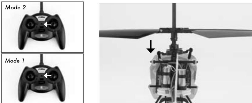
With the stick pushed right, the left-hand servo should push the swashplate upward.
