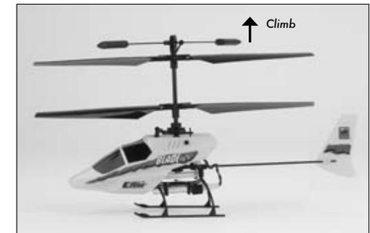
Decreasing the speed of the main rotor blades by lowering the throttle stick will cause the model to descend.
