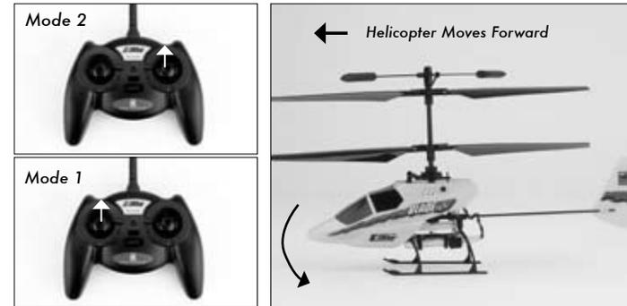
Pulling the stick backward will pitch the tail of the helicopter downward, allowing the helicopter to be flown backward.
