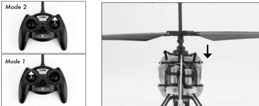
With the stick pulled back, the right-hand servo should push the swashplate upward.
