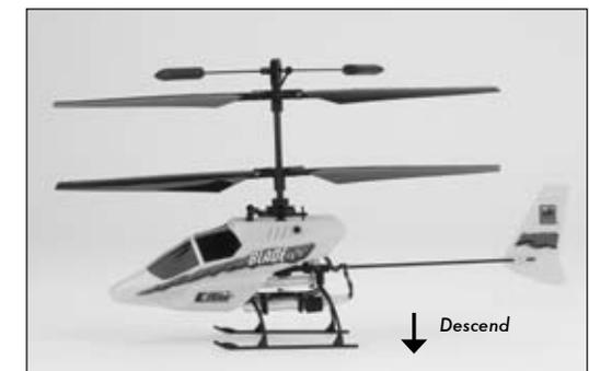
After lifting the model off the ground you can balance the throttle by carefully moving the throttle stick up and down so the model will hold a stationary hover without climbing or descending.
