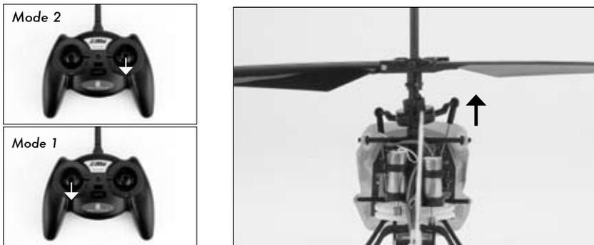
Move the right-hand stick left and right to check aileron roll control. When the stick is pushed to the left, the left-hand servo (when viewing the helicopter from behind) should pull the swashplate downward.
