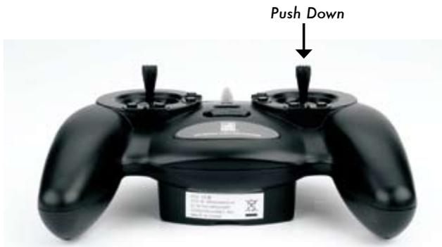
When the transmitter is first powered on it will be in the high rate mode. You can tell you are in the high rate mode when the LED on the transmitter glows solid red. In the high rate mode the controls are allowed to reach their maximum values, which is typically preferred by experienced pilots interested most in maximum control authority.
