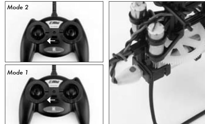
Move the elevator stick on the transmitter forward and aft to check elevator pitch control. When the stick is pushed forward, the right-hand servo (when viewing the helicopter from behind) should pull the swashplate downward.
