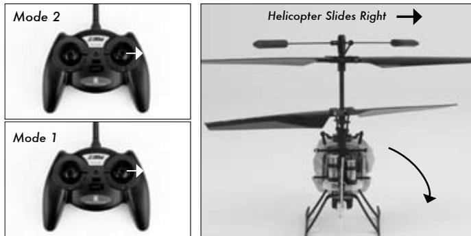
The aileron trim can be used to help keep the helicopter from drifting left or right when in hover with no aileron stick input. For example, if the helicopter drifts to the right when in hover, add left aileron trim until the helicopter hovers as level as possible with no drifting to the right.
