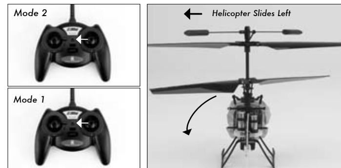
Moving the aileron stick to the right will roll the helicopter to the right, allowing the helicopter to be flown to the right.
